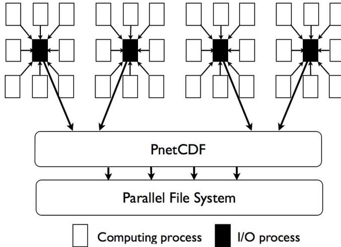
**Fig. 2.** The schematic diagram of the I/O forwarding technique.
