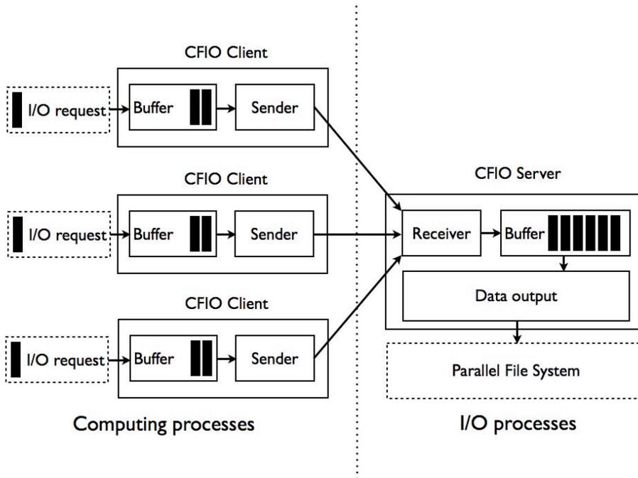
**Fig. 3.** The system architecture of CFIO.
