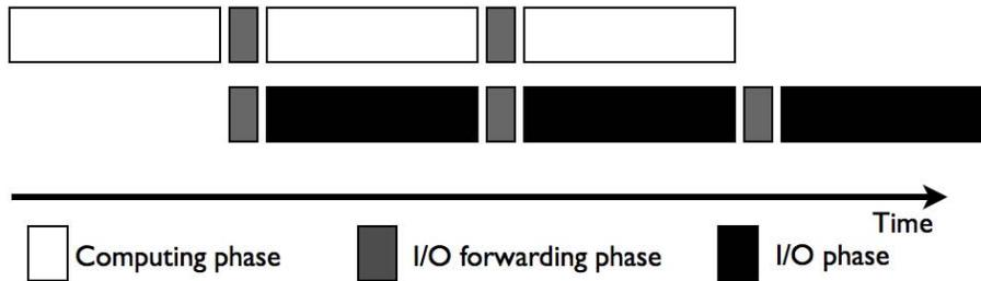
**Fig. 4.** Overlapping I/O with computing through I/O forwarding.
