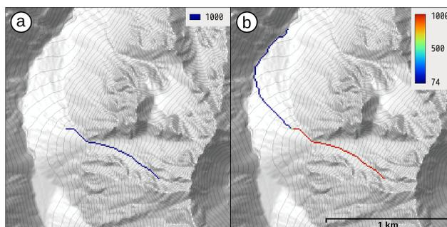
**Figure 5.** Sink filling; (a) the process stops in a sink; (b) the process overcomes the sink and stops in the next sink because no material is left over.
