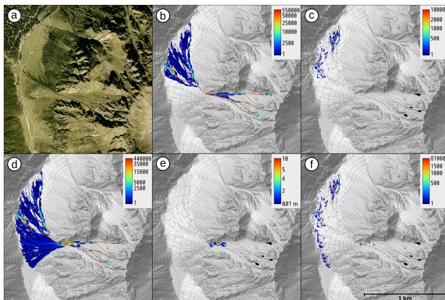
**Figure 8.** Deposition modeling scenario on a high resolution 2.5 m DTM; (a) orthophoto, (b) transition frequencies (no deposition), (c) stopping positions (no deposition), (d) transition frequencies (deposition), (e) material deposition heights, (f) stopping positions (deposition). For details see text.
