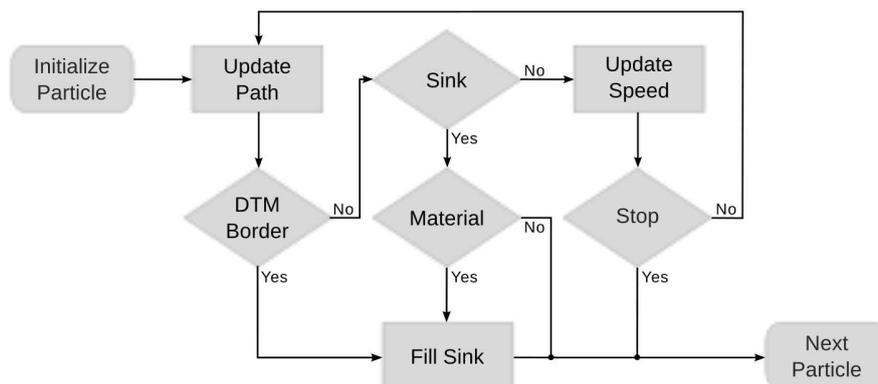
**Figure 2.** Flowchart of a GPP model configuration making use of the sink filling approach.
