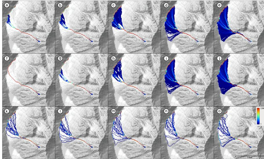
**Figure 4.** Effect of different random walk parameter settings; (a) to (e): different exponents for divergent flow (1.0, 1.1, 1.2, 1.5, and 2.0); (f) to (j): different slope thresholds (15°, 20°, 30°, 40°, and 60°); (k) to (o): different persistence factors (1.0, 1.5, 2.0, 2.5, and 3.0). For details see text.
