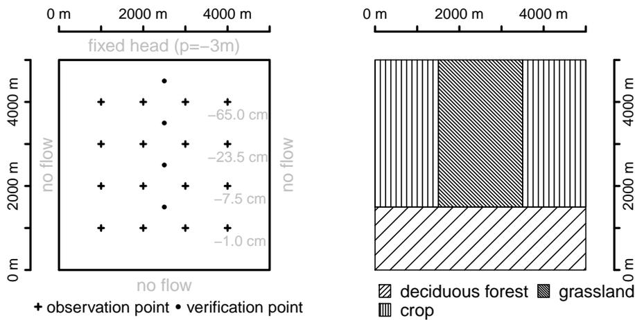
**Figure 5.** Synthetic setup for the twin experiment. The left hand figure shows boundary conditions of the subsurface model (ParFlow) and the location of observation (crosses) and verification (filled circles) points. Grey numbers indicate the depth of observation and verification nodes which are constant in W-E-direction. The right hand figure shows the spatial distribution of plant functional types used in the land surface model (CLM).
