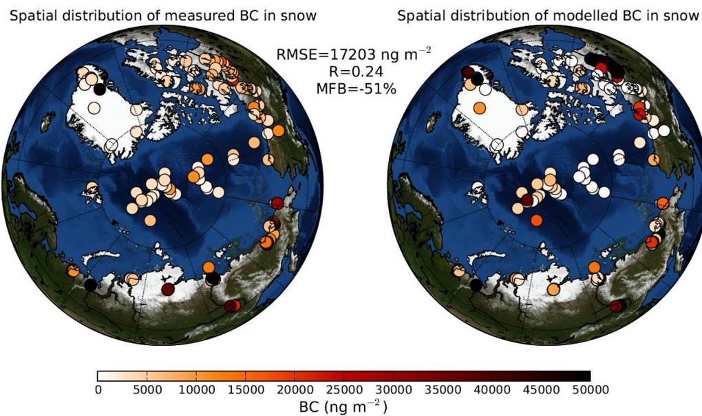
Figure 7: Measured and modelled BC concentration in snow.
