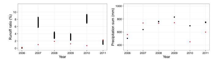
**Figure A1.** Comparison of simulated yearly runoff coefficients (left) and precipitation forcing (right) for all 12,250 discretisations (black dots) with values reported by Medeiros and de Araújo (2014) (red dots).
