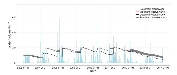
**Figure 4.** Time series plot of daily resolution of simulated (all 12,250 parameter realisations) and observed Benguê reservoir volume and areal precipitation. Note that the maximum reservoir level corresponds to the official value which has been used for model parameterisation. Observations sometime show slight deviations due to, e.g., random measurement errors or changed rating curves.
