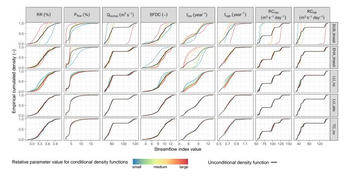
**Figure 7.** Unconditional (black lines) and conditional (rainbow coloured lines) empirical cumulative distribution functions for each streamflow index—discretisation parameter combination.
