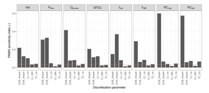
Figure 6. Barplots of PAWN sensitivity indices  $T_j$  for each streamflow index and landscape discretisation parameter. Red lines indicate critical Kolmogorov-Smirnov values ( $KS_{crit}$ ), i.e., parameters, for which  $T_j$  is not greater than this value, can be regarded as insignificant for the respective streamflow index.
