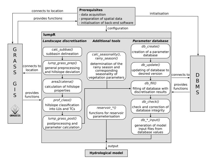
**Figure 1.** Schematic overview of the functionalities of the lumpR package. Shown are all available functions (*in italics*) with a short explanation, interactions with external components, and the typical flow of information during the application. Note that the acronym DBMS refers to *DataBase Management System*.
