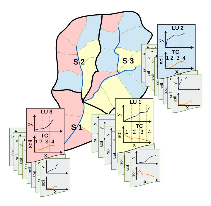
**Figure 2.** Example of the outcome of steps (i) to (iv) of landscape discretisation. Shown is a hydrological basin sub-divided into subbasins (labelled S 1–3), EHAs (green outline), and LUs (red, blue, yellow) with TCs. Along-slope catena properties for the EHAs and LUs are summarised by the diagrams.
