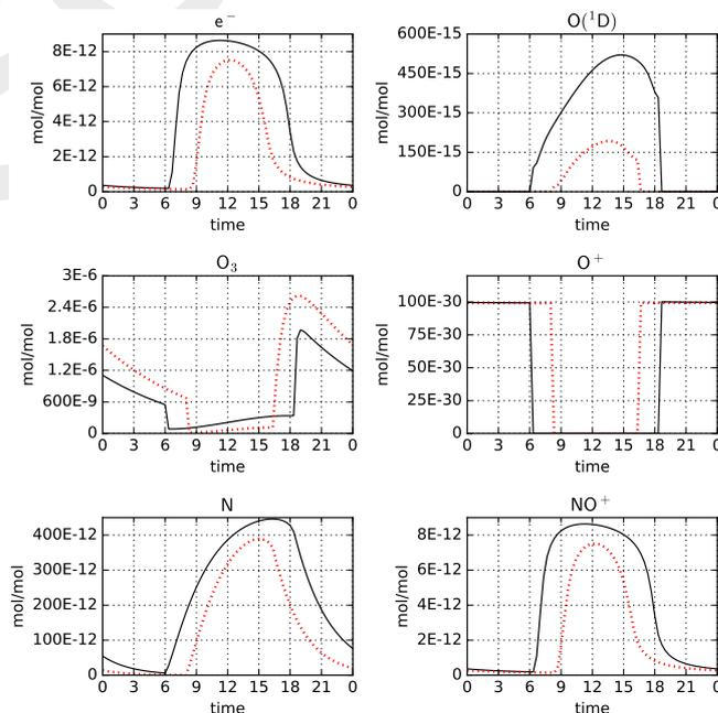
**Figure 5.** Model-calculated mixing ratios from an upper atmosphere simulation with MECCA and RADJIMT: Diurnal cycles for 4 January (after 3 days of spinup) for the equator (black) and a latitude of 50° N (red). Time is in hours, with local noon at 12. See Sect. 3.2 for further details.
