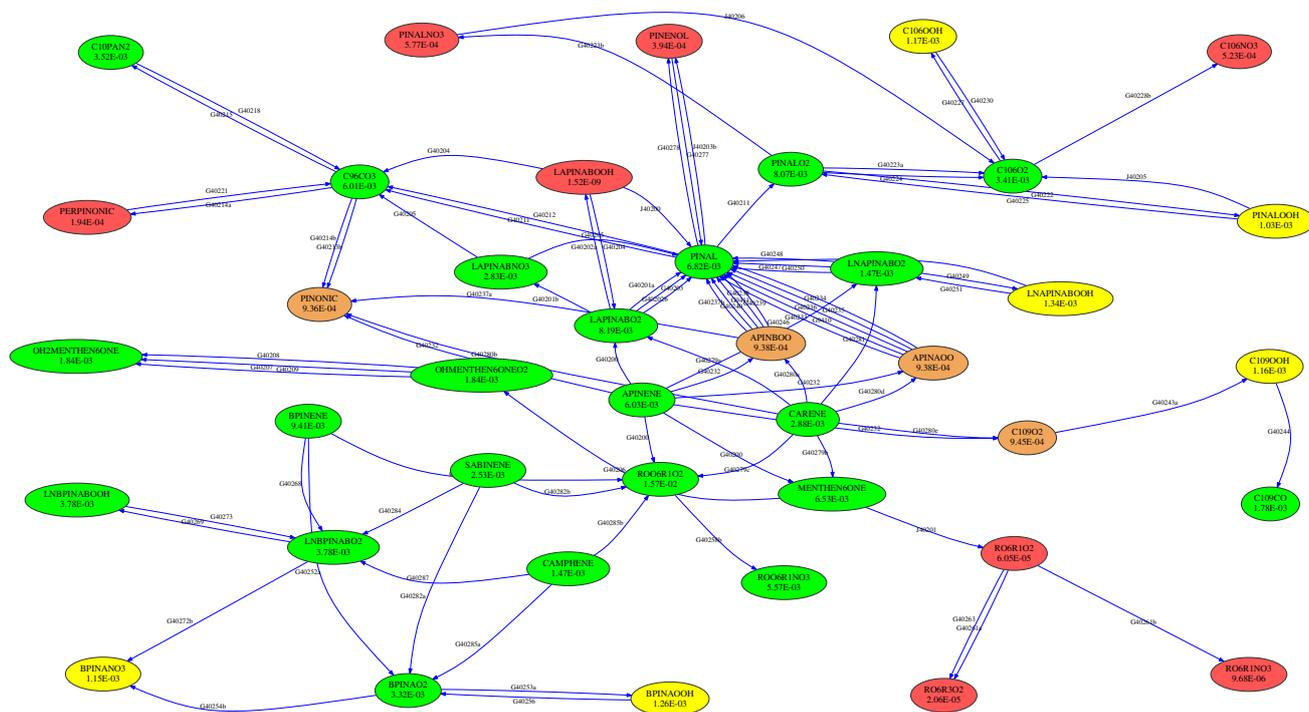
**Figure 4.** Skeletal reduction of terpene chemistry in the MOM reaction scheme (only  $C_{10}$  species are shown here). Vertex colors and OIC values correspond to those in Tab. 3: Only the green and yellow species are kept in the reduced mechanism.
