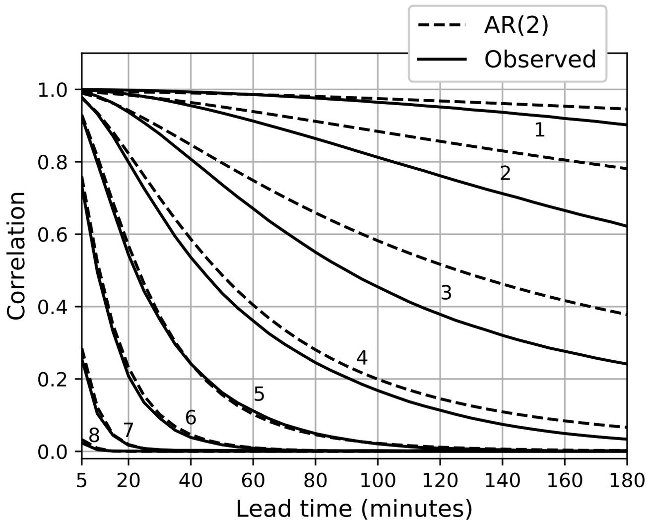
**Figure 10.** Temporal auto-correlation estimates obtained from AR(2) models (dashed lines) and the correlation between an extrapolation nowcast and the corresponding observations. The analysis is based on the FMI events (Table 7). The line numbers correspond to the frequency bands shown in Fig. 1 from left to right.
