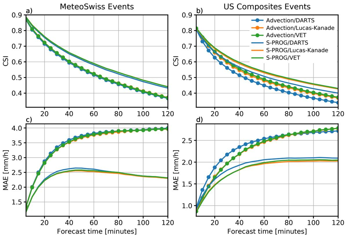
**Figure 11.** Comparison of forecast skill using different optical flow and extrapolation methods. The left panel shows the averaged CSI and MAE for the MeteoSwiss events listed in Table 8, while the right panel shows the same results but for the US events listed in Table 9.
