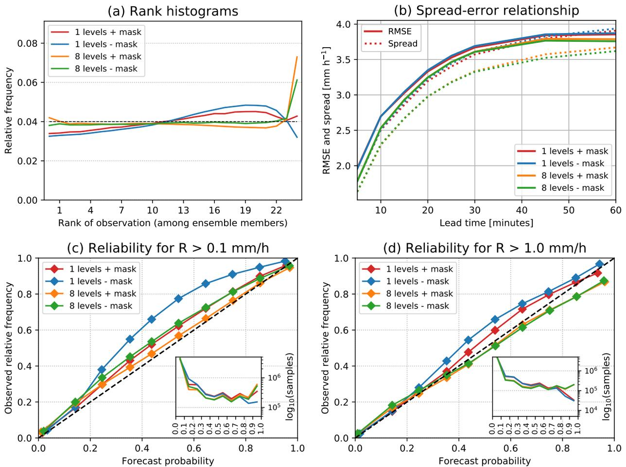
**Figure 19.** Ensemble and probabilistic verification of the cascade experiments for all the MeteoSwiss cases with and without cascade decomposition, and with and without masking. a) Rank histograms at 60 min, b) spread-error relationship, c,d) reliability diagrams at 60 min for probability of rain exceeding 0.1 and 1  $\text{mm h}^{-1}$  respectively.
