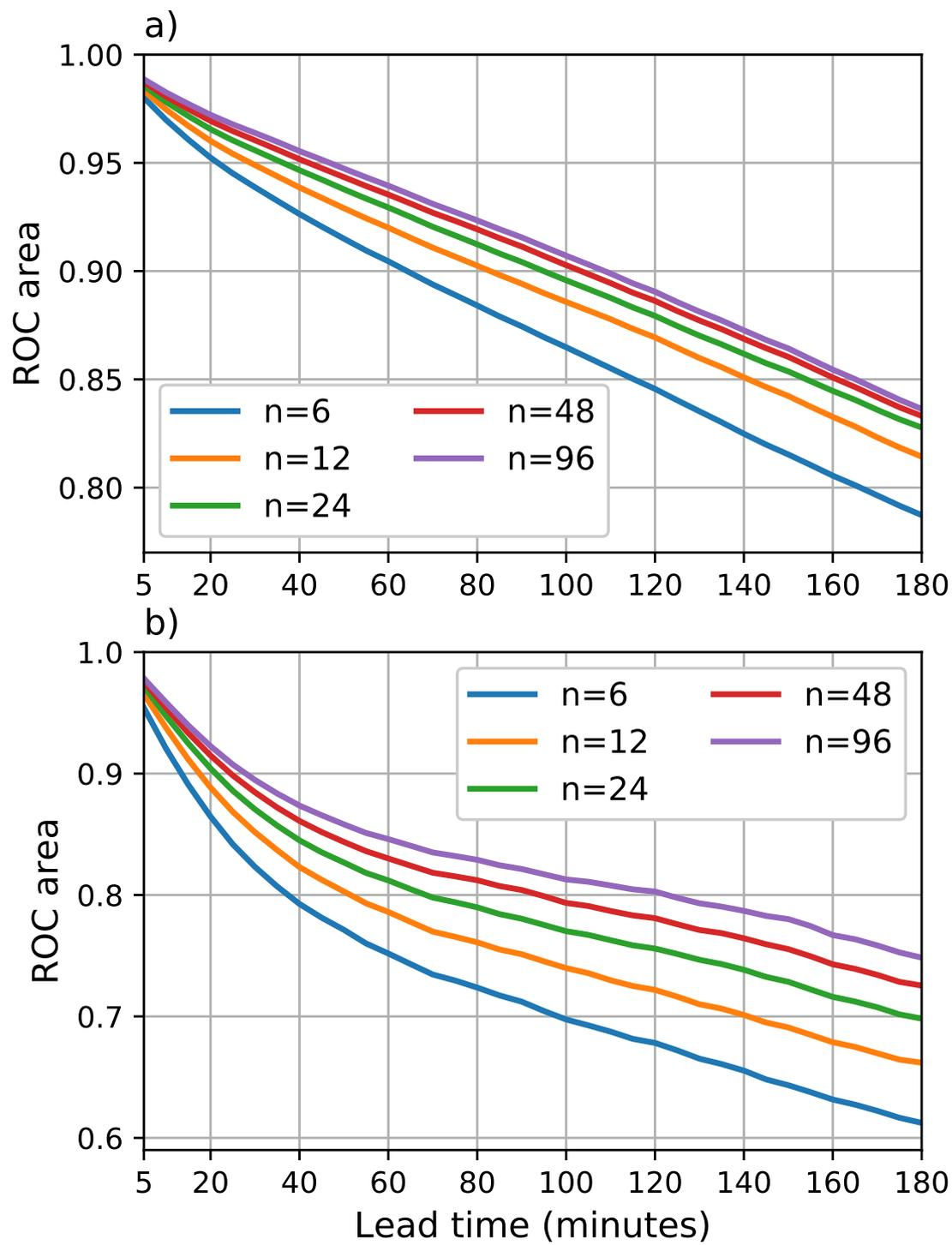
**Figure 13.** ROC areas for (a) 0.1 mm h<sup>-1</sup> and (b) 5 mm h<sup>-1</sup> thresholds with different ensemble sizes as a function of lead time during the MeteoSwiss events listed in Table 8.
