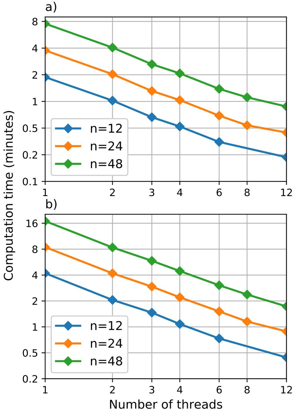
**Figure 15.** Averaged computation times of pysteps nowcast ensembles with different ensemble sizes and number of parallel threads for the (a) MeteoSwiss and (b) FMI domain. The grid sizes for the domains are 710x640 and 760x1226 pixels, respectively. One-hour nowcasts with 12 time steps of 5 minutes were computed for both domains. The computation times include only the ensemble computation, excluding the optical flow, the initialization of the model and writing the results to disk.
