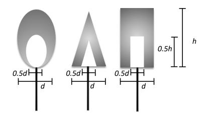
**Figure 1.** Representation of the individual crowns and stems. The tree crown objects are defined as either cone, cylinder, or spheroid, where d is the maximum diameter of the object and h is a crown height. The crown objects are divided by two domains. Outer domains (grey colored domains in the figure) are filled with green leaves. Inner domains are filled with woody materials. In the default setting, the size of inner domains are set as half of the crown size.
