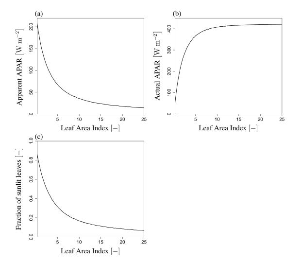
Figure 16. Variation of apparent and actual APAR and fraction of sunlit leaves with respect to LAI. (a) Apparent APAR, (b) Actual APAR, and (c) Fraction of sunlit leaves at SZA= $20^{\circ}$ . These variables are not affected by the view direction. APAR<sub>app</sub> and F<sub>sun</sub> decrease exponentially and APAR<sub>c</sub> increases and then becomes saturated with an increase in LAI.
