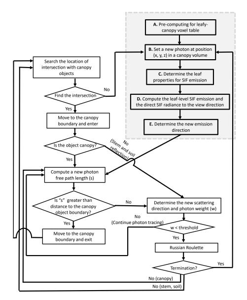
**Figure 2.** The flowchart of the Monte Carlo photon tracing scheme in canopy landscapes at a single-wavelength. The procedures A to E framed by the dotted grey rectangle indicate the photon tracing scheme for direct SIF emission. The other part of the flowchart corresponds the multiple scattering. The multiple scattering schemes are the same as the original FLiES model (Kobayashi and Iwabuchi, 2008).
