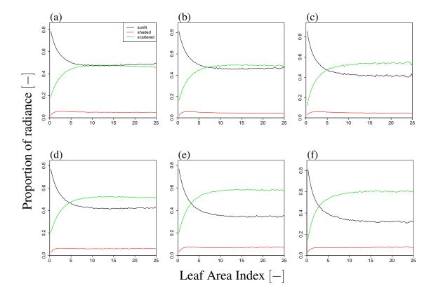
**Figure 15.** Proportion of SIF radiance in LAI variation. Upper figures (a)–(c) and lower figures (d)–(f) indicate results in forward and backward directions, respectively, for different VZA values  $(10^{\circ}(left), 30^{\circ} (center), and 50^{\circ} (right))$ . The contribution of shaded leaves is small and the contribution of scattered radiance increases with LAI and VZA. Additionally, in the backward direction, the contribution of scattered radiance increases with LAI and VZA.
