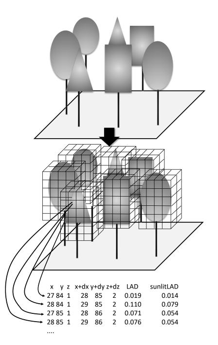
**Figure 3.** Voxel extraction from geometric canopy landscapes. The leaf voxel is extracted before the ray tracing simulation. FLiES-SIF model uses the geometric object approach for the Monte Carlo ray tracing. For the SIF simulation, the ray tracing is initiated from the randomly selected positions in the forest landscape. This voxel information is used to efficiently select the leaf position where SIF occurs.
