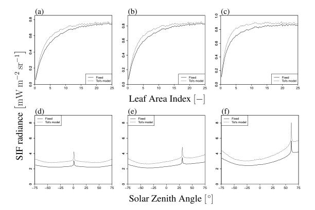
**Figure 17.** Comparison of SIF radiance with different  $\phi_f$  (constant and from Tol's model). Upper and lower figures indicate SZA dependency (LAI = 3.0) and LAI dependency (SZA=20°), respectively. The VZA values are 0° (**a** and **d**), 30° (**b** and **e**), and 60° (**c** and **f**). The solid line indicates the case of constant  $\phi_f$  (=0.01). The dashed line indicates the result of Tol's model, where  $\phi_f$  depends on APAR<sub>L</sub>, as shown in Fig. 7.
